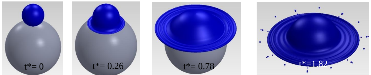
(b) 2D-front view of splash regime: We=520/TP=140^\circ C
