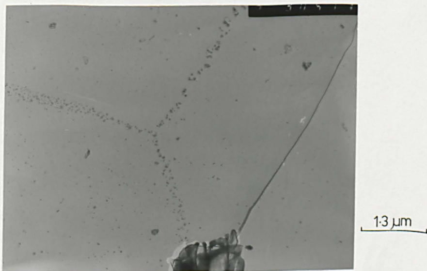
Fig. 6.11 C-Mn-Al steel heated directly to 850°C, showing grain boundary precipitation of AlN.
