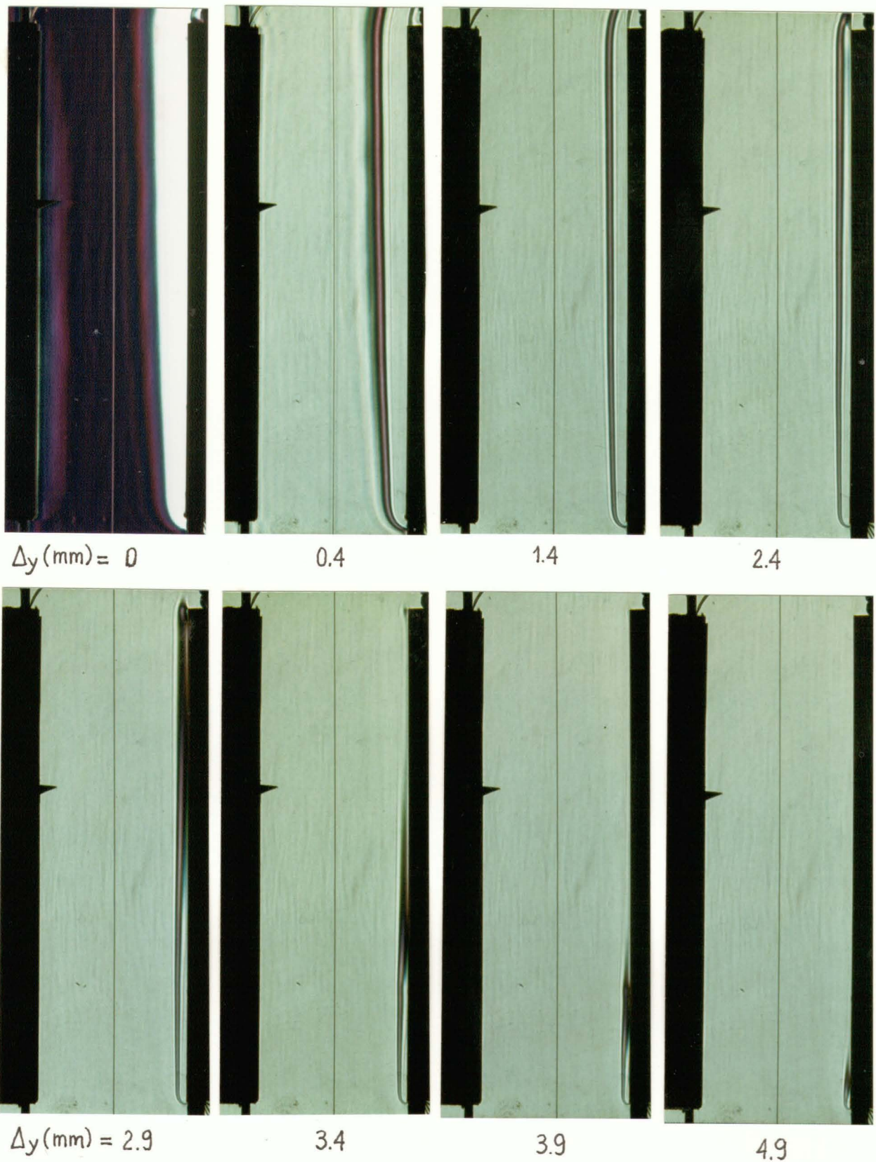
FIGURE 4.14 Schlieren images (focal filament method) of the smooth channel configuration, filter mounted vertically, Ra=1.8 \cdot 10^7 , S/H=0.3 . \Delta_y from 0 (top left) to 4.9 mm (bottom right).
