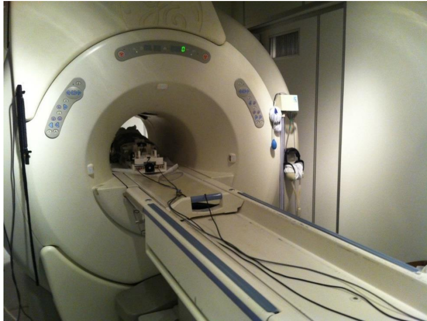
Figure 5.1: Photograph of the 1.5 T GE Signa Excite HD MRI system used for guiding HIFU thermal exposures of the designed tissue mimicking phantoms.
