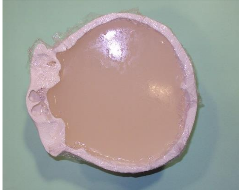
Figure 4.9: Finalised composite head phantom.
