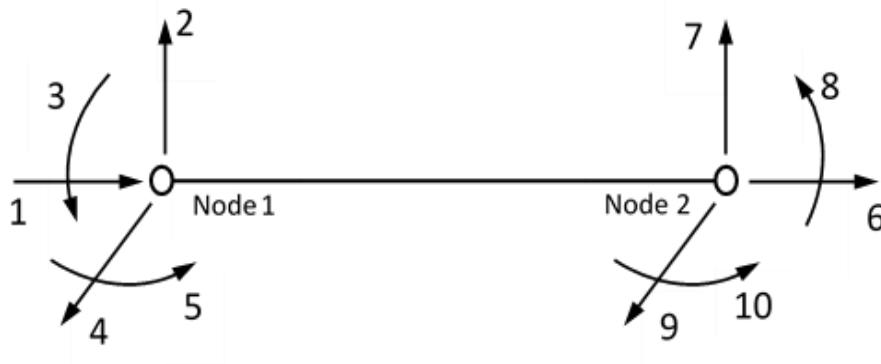
Figure 5.13: Element degrees of freedom in global system.
