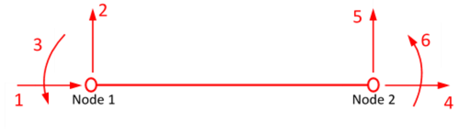
Figure 5.14: Element degrees of freedom in local system for longitudinal member.
