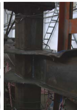
(e) Buckling of beam in joint C
