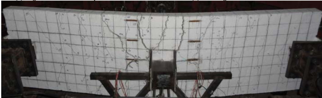
(c) cracking pattern at top of slab
