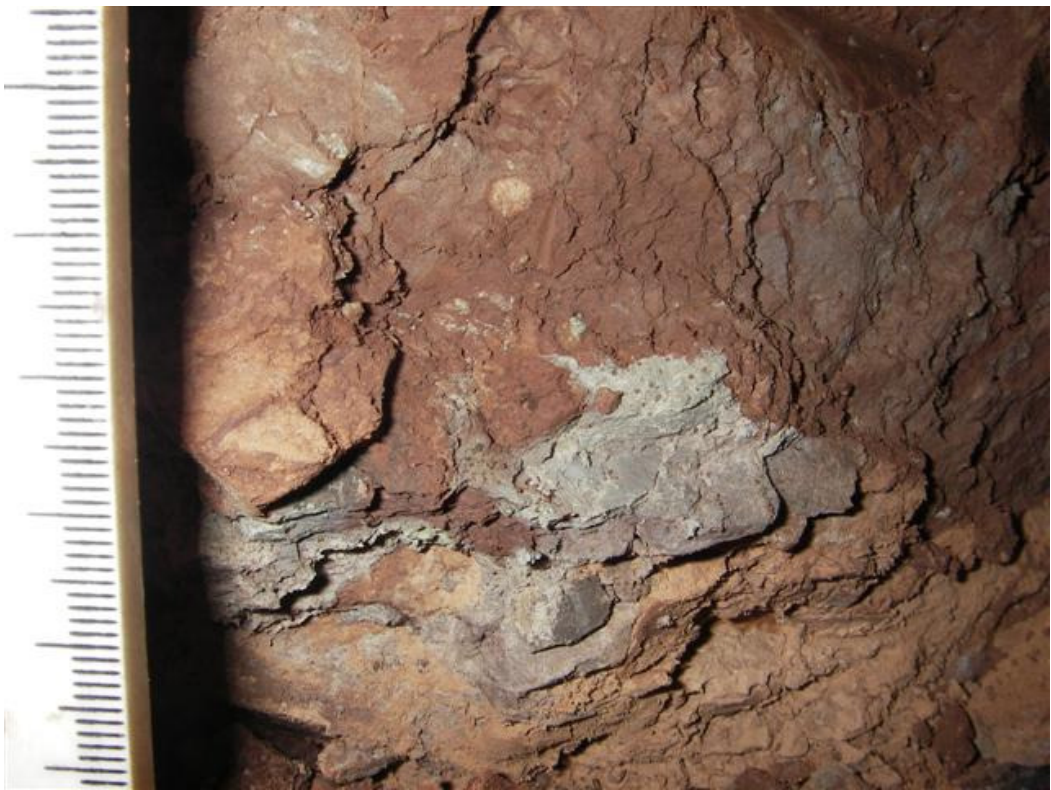
Figure 4.23 Vertical section with green mottling within the remoulded zone around pile MR2, at a depth of 1547mm below ground level
