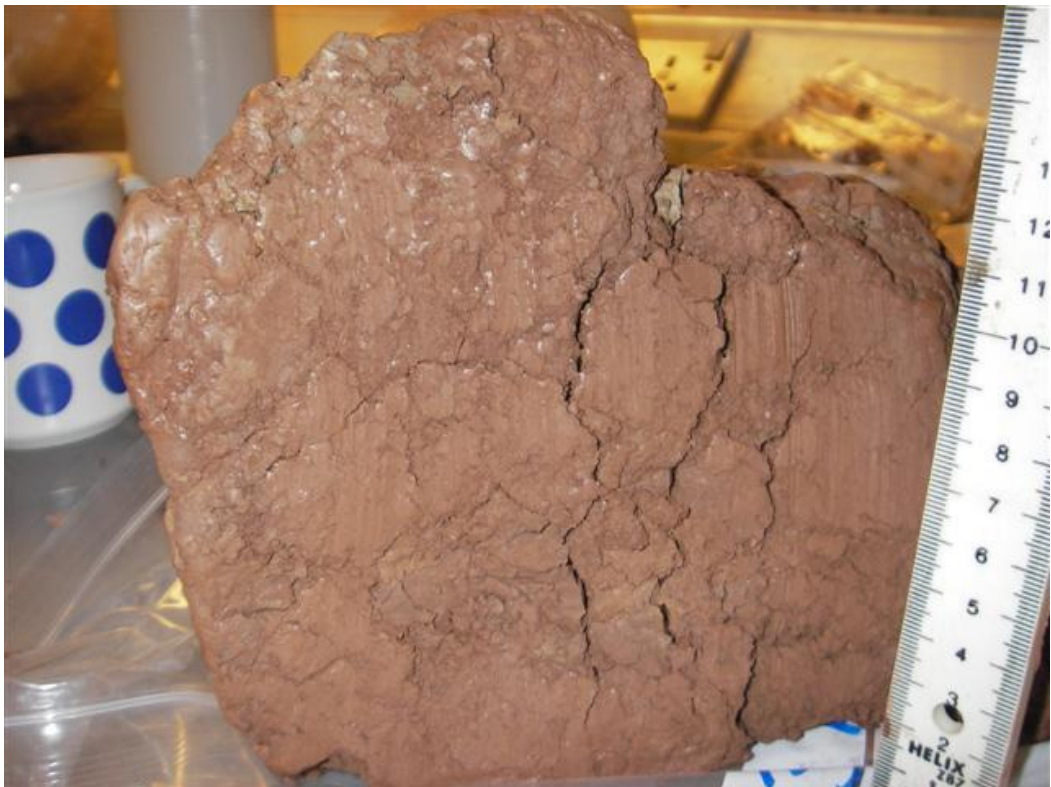
Figure 4.34 Te inner surface of the remoulded zone from around pile MR3, 860-1210mm below ground level. Pile would have been to the front of the picture
