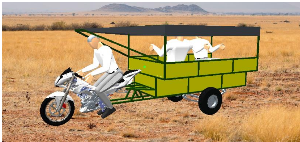
Figure 5: Concept of 3-wheeler adaptation of a motorcycle
