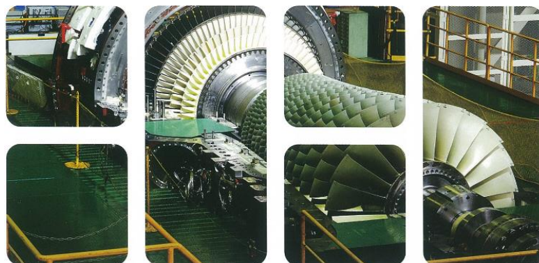
Figure 1.2: J-series gas turbine developed by Mitsubishi Heavy Industries, Ltd [3].
