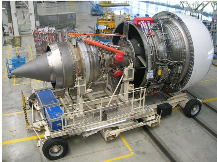
Figure 1.3: Rolls-Royce Trent 900 engines, Type: Turbofan [4].
