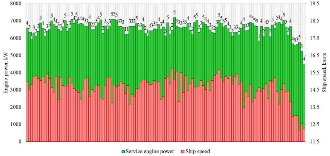
Figure 12.2 Measured ship service engine power and ship speed observed.
