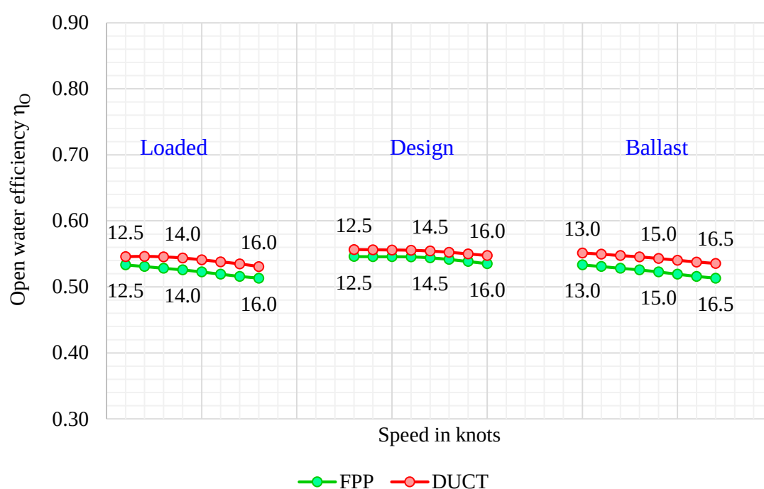
Figure 7.18 The comparison results of the propeller efficiency of the 19A ducted propeller (DUCT) and the conventional fixed pitch propeller.
