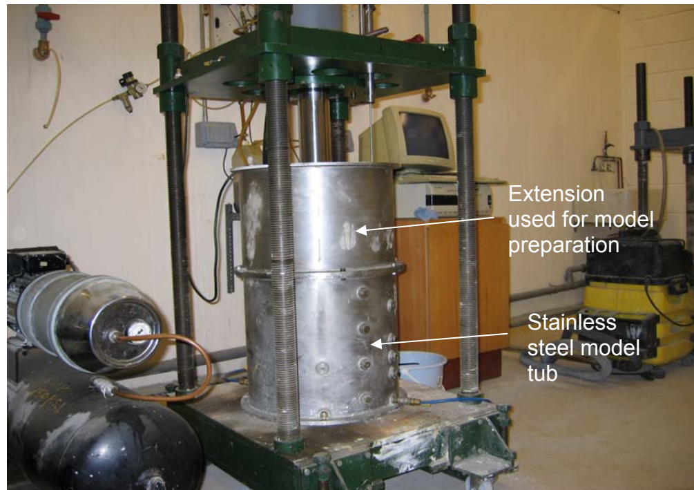
Figure 3.39 Stainless steel model tub and extension used for centrifuge model preparation.
