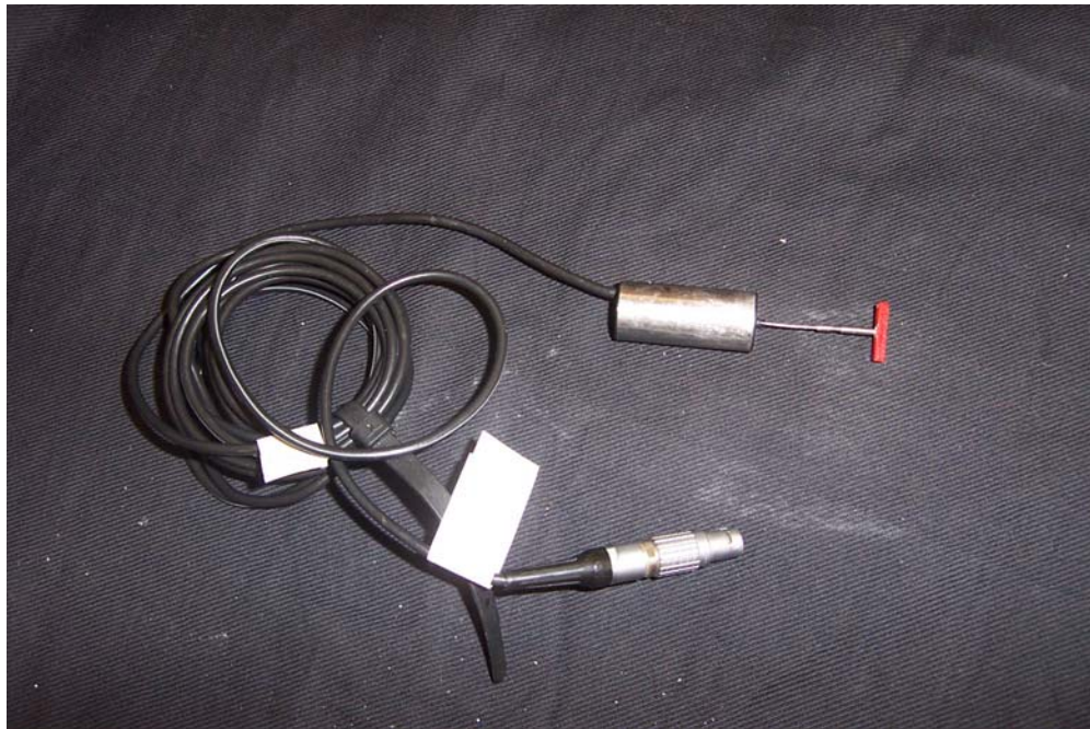
Figure 6.7 LVDT used to measure model pile displacement during centrifuge testing.
