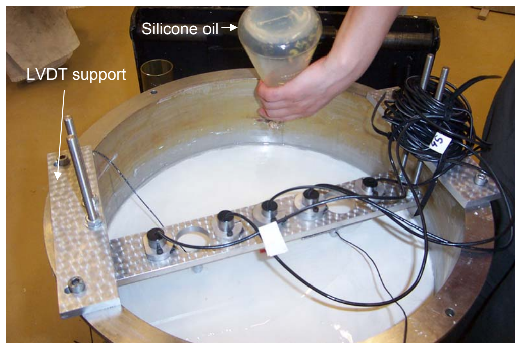
Figure 3.61 The model clay with an impermeable surface sealed with silicon oil.
