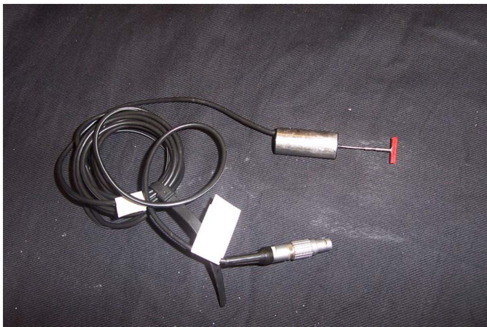
Figure 4.4 LVDT used to measure model pile displacement during centrifuge testing.
