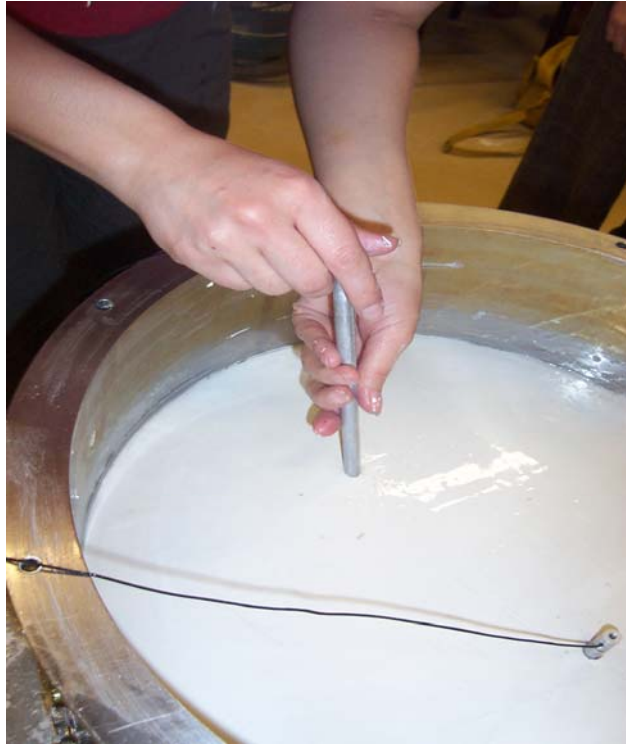
Figure 6.3 Installation of 10mm diameter model piles at 1g.
