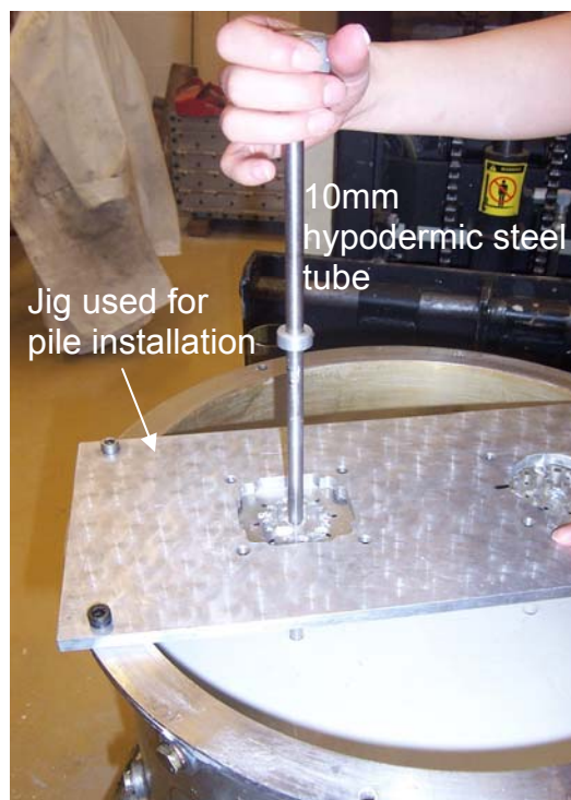
Figure 3.48 Model pile installation at 1g using a template to position and install piles.
