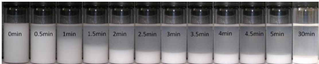
Fig. 2.2 A gravity settling experiment of 0.5 wt% \text{Al}_2\text{O}_3 /water (Witharana et al., 2012)
