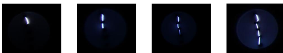
Figure 17. The discharge images for actuator with different number of discharge channels (the discharge channel increases from one to four from left to right)
