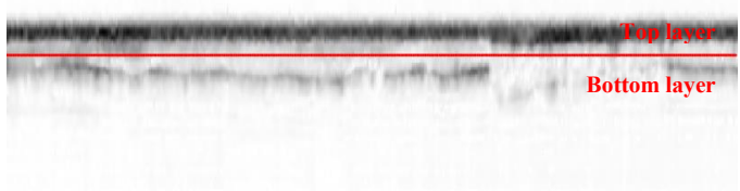
Figure 5. GPR processing example: division into layer regions
