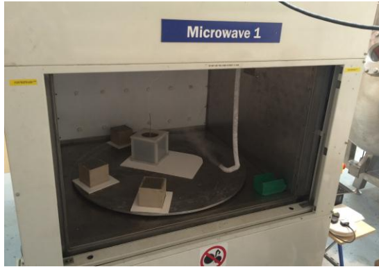
Fig. 8 Scaled-up trial of microwave-cured concrete
