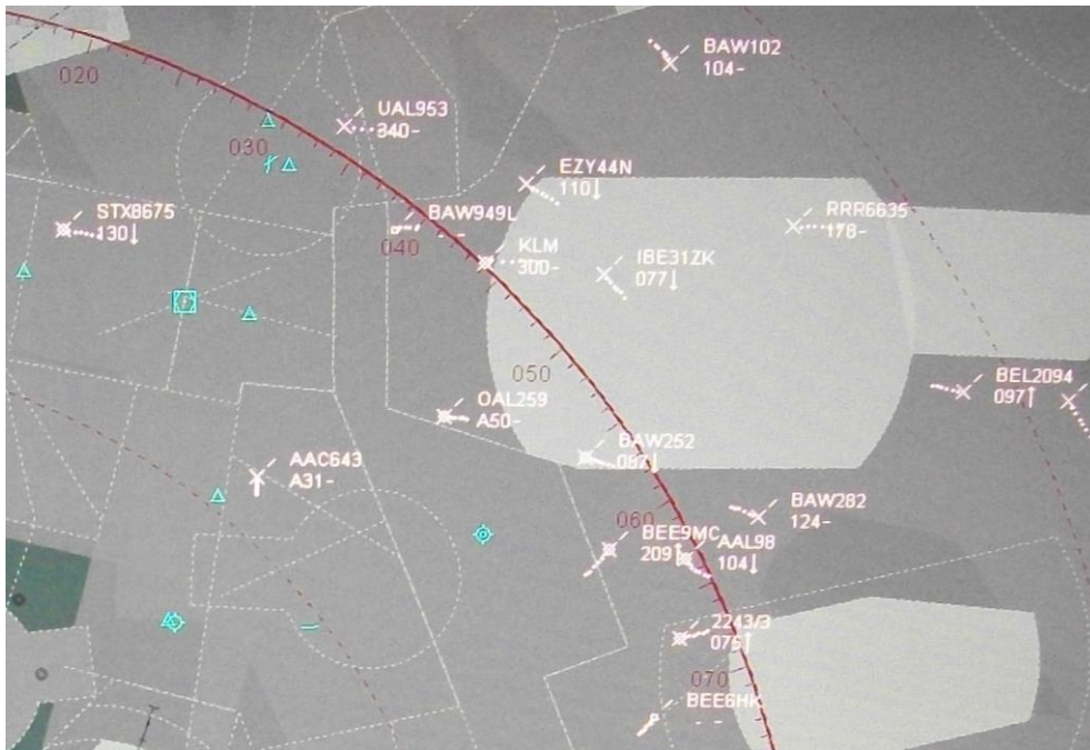
Figure 2: Example of colour coded data blocks used in air traffic control. Data blocks are clusters of small text containing descriptive information of a flight and altitude, the colour indicates whether they are owned or not and whether there are any warnings associated with a particular aircraft.
