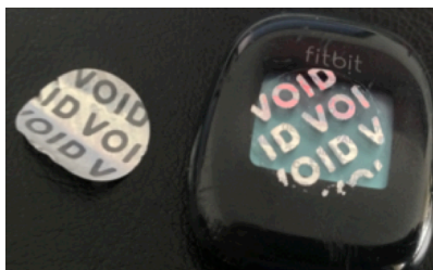
Figure 2: The Fitbit Zip activity tracker, showing a removed tamper-evident sticker. The sticker was applied to all devices used in groups 1 and 2, immediately after set-up. Each sticker was printed with the participant number to prevent participants replacing the sticker.
