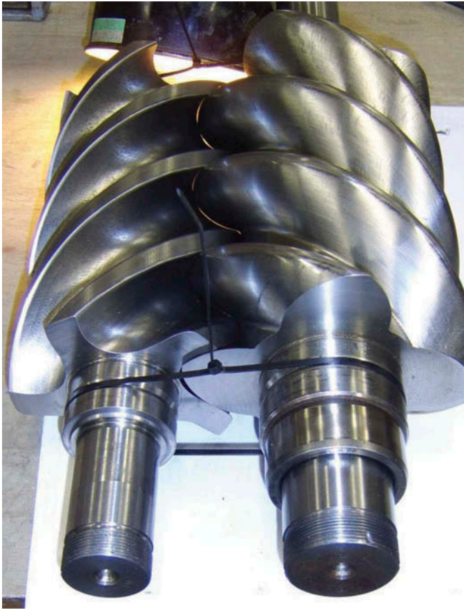
Fig. 6. Optimized screw expander rotors for wet steam application.
