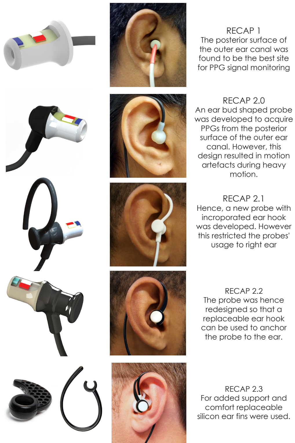
FIGURE 7.16: A flowchart of 3D models and photographs illustrating the incremental design and development of the RECAP PPG probe.
