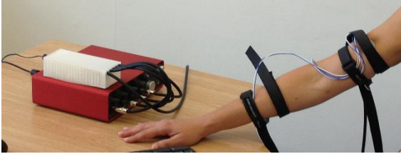
Figure 1: Overall setup of the hardware. Left: the audio interface (red box) with the circuitry for the acoustic myograph (white box). Right: the placement of the four sensor units on the arm.
