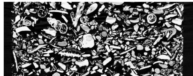
Fig. 8. Tomographic image of coarse carbonate sand, taken before thermal cycling, showing the presence of large voids within the material
