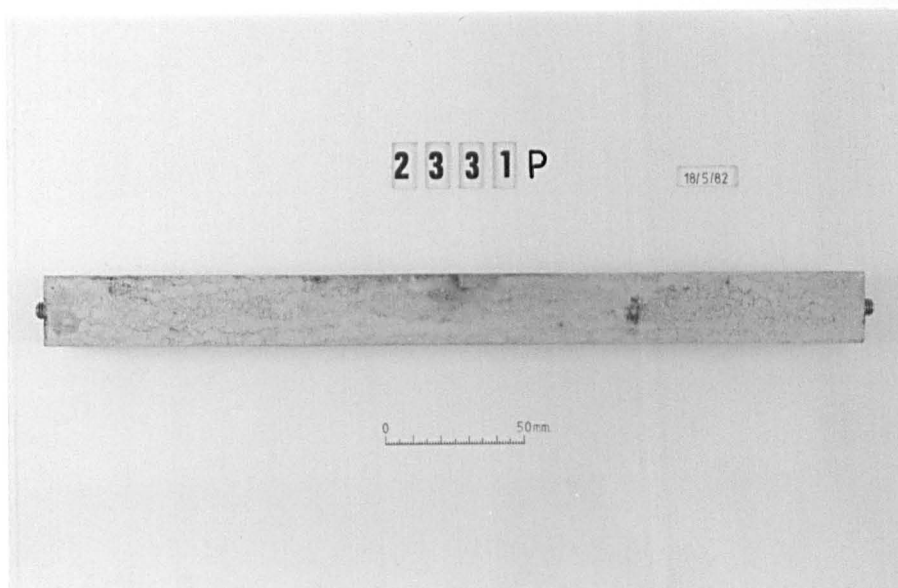
Plate 6.9 Mix Ref. 2331P, showing the surface condition of a typical mortar bar subsequent to the expansion measurement taken at age 6 months.
