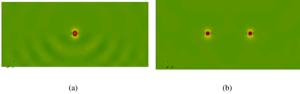
Fig. 10.5 (a) H_y field profile propagating in the nano input wire, (b) H_y field profile after splitting the input power into two at the output nanowires
