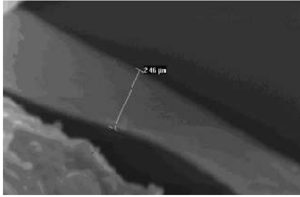
Figure 5 shows the voids (black lines) between the fibres and epoxy. The white line is 2.46 \mu\text{m} long
