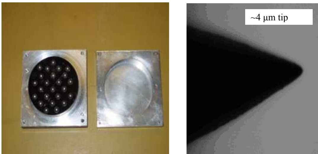
Figure 1 (a) Mould for multiple recessed specimens, (b) electrolytically etched needle
