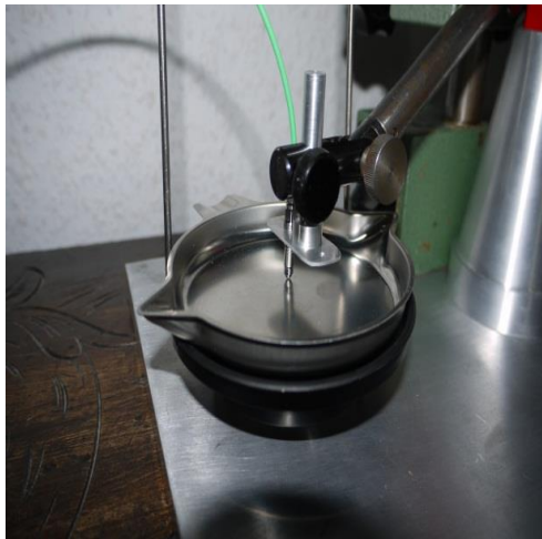
Figure 5.10 Calibration of the low force sensor.
