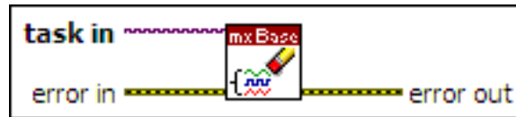
Figure 9.15: Diagram of DAQmx Base Clear Task VI.
