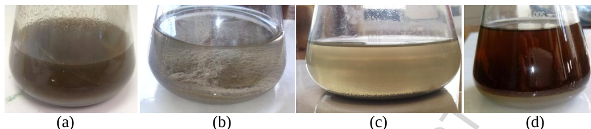
Figure 2: Visual characteristics observation is a direct way to see the effect of solvent and stirring time: 2wt.% GO-Al dispersion with stirring time of (a) 1 h in acetone, (b) 5h in acetone, (c) 5h in ethanol-water, and (d) 5h in ethanol.
