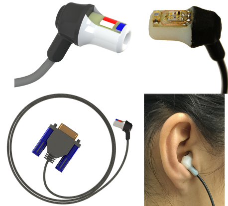
Fig. 2: 3D model and photographs showing the ear canal PPG probe.
