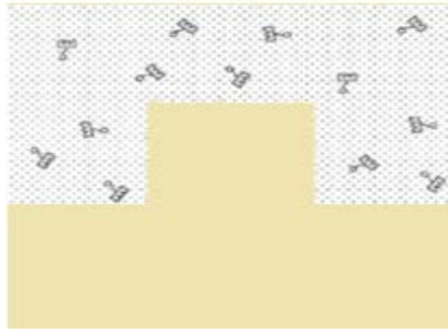
Figure 2.11: Homogeneous sensing where analytes exist in the surrounding aqueous medium that serves as the top cladding [127].
