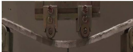
Fig.3. High flexural deformation of SHCC
