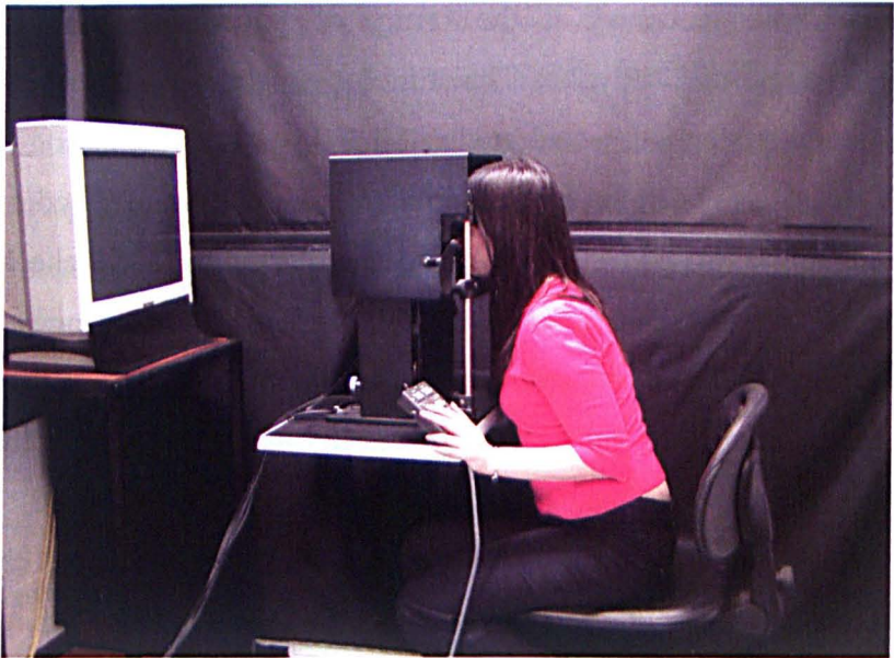
Figure 3.6: Photograph of experiment set-up. The headrest facilitates fixation and ensures the viewing distance is 700 mm. The response button box is also shown; the subject presses one of the four buttons according to the direction of motion of the stimulus.
