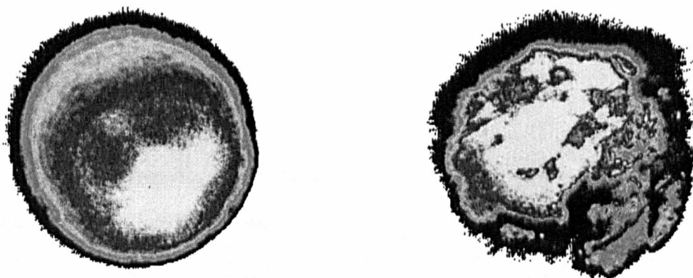
Fig. 5-2: Intensity-profiles at the endface of a capillary, filled with air (left) and water (right)
