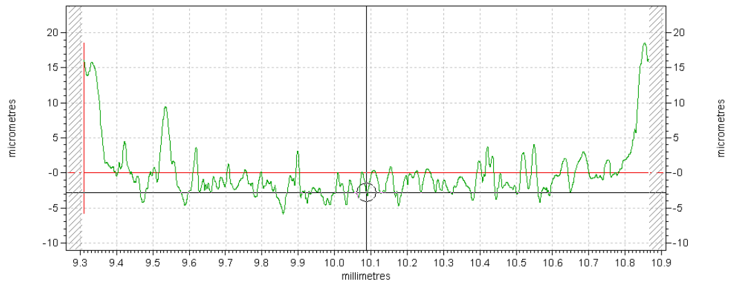
Figure 3.16: Profile measurement around the area of laser path
