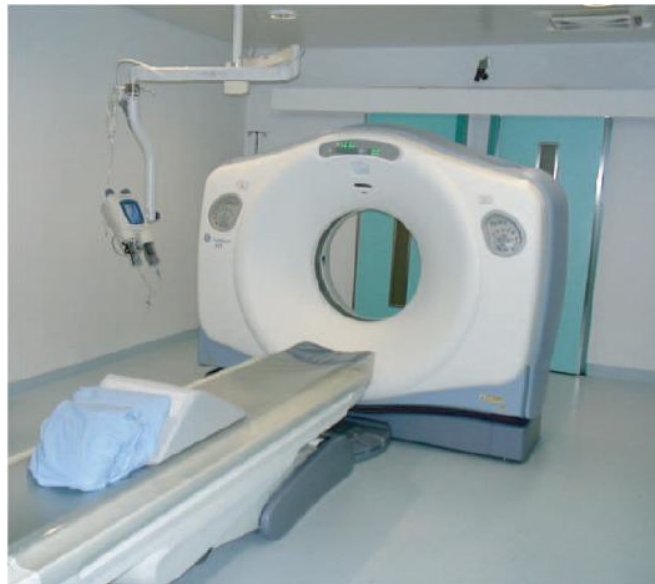
Figure 1.5: A modern multiple slice Computed Tomography machine. The patient is placed on the table, moving through the ring unit, which is comprised of the X-ray source and the detector [5].
