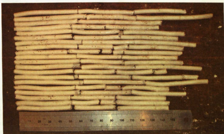
Figure 5.09 Spoil from clay coring: three cuts per pile (test 3b)
