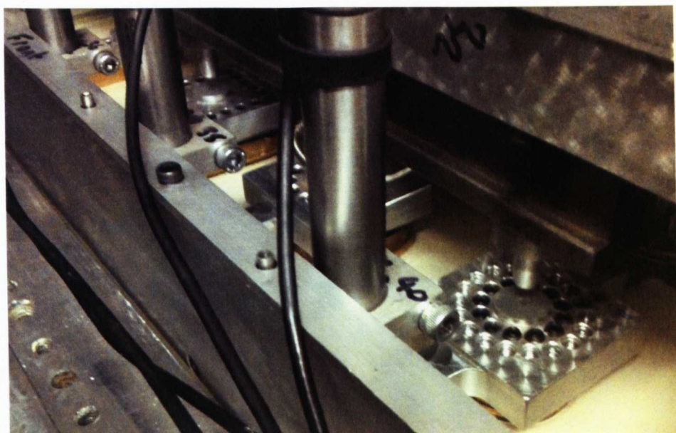
Figure 5.18 Loading beam and load cell in place above loading point and pile cap (test 5d)
