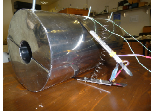
Figure 6.8 Deflecting strain gauge on lagging
