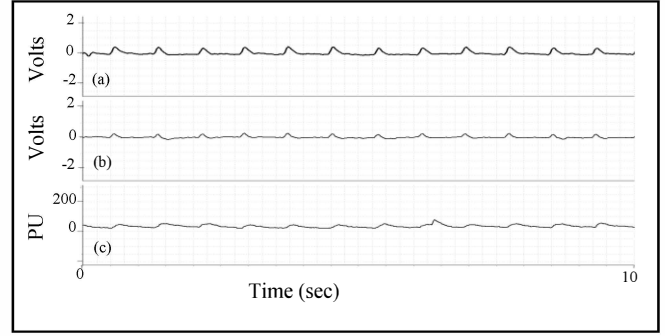
Figure 4. (a) IR_{AC} , (b) R_{AC} and (c) laser Doppler signals at 75 mmHg for 10 second.
