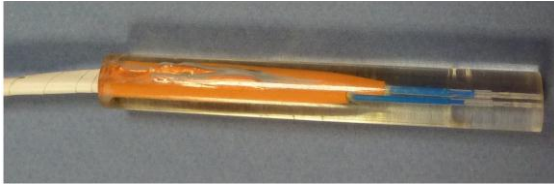
Fig.2. Splanchnic pulse oximetry fibre optic probe
