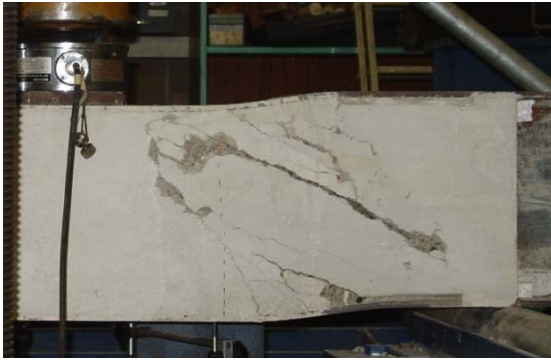
Figure 9. USFB No.3 at Failure point.
