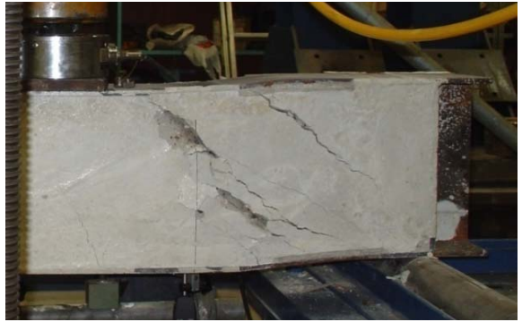
Figure 10. USFB No.4 at Failure point.
